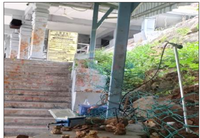
9. GROUND VIBRATION MONITORING AT THE TEMPLE
