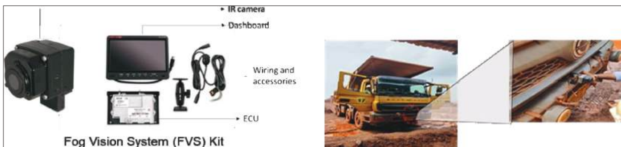
Fig. 10: Components of Fog Vision System (left) and its installation on Bharat Benz dump truck
