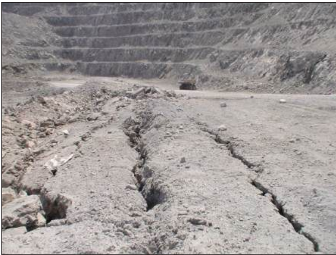
4. Trend of blast induced back-break
